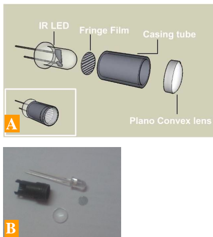
Figure 1. A)Exploded view of nano-projector B)parts of nano-projector
